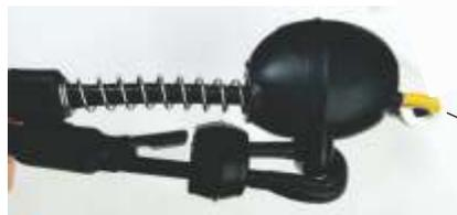
Automatic quick release safety system, disengages the cable it is being pulled by.
